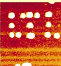
7) Steps 2-6 or 1-6 may be iterated to arrange the particles at the desired positions.
