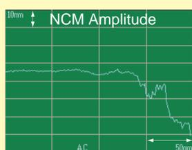
6) After lowering the tip some nanometers more, the particle has moved as is obvious in the **NCM amplitude** data.
