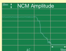
5) The tip is lowered until plateau start to be visible at the position of the particle in the **NCM amplitude** data.
