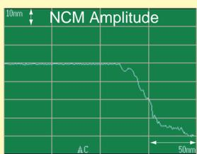
4) Feedback-loop is turned off and **NCM amplitude** is acquired from the scanned line. The particle is visible in the data.
