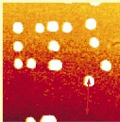
1) Topography image of the sample surface is taken in NCM to locate the particles.
