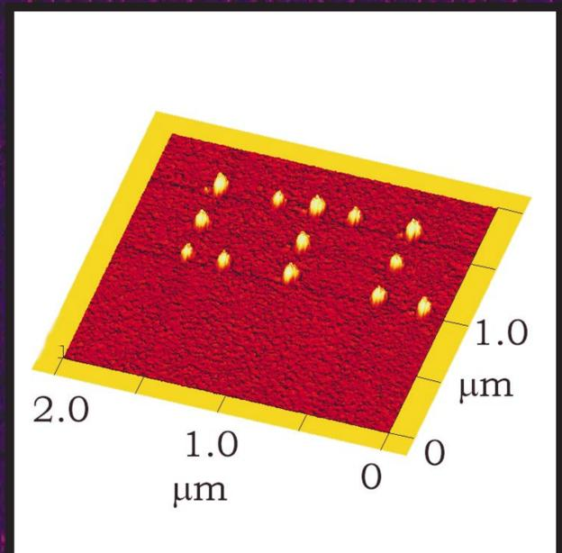
**Figure 2:** "LTL" (Low Temperature Laboratory) written in block letters using 45 nm silver particles.
