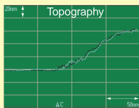
3) The exact position of the particle is found by looking the **topography** of the line scan and by varying the line scan position slightly.
